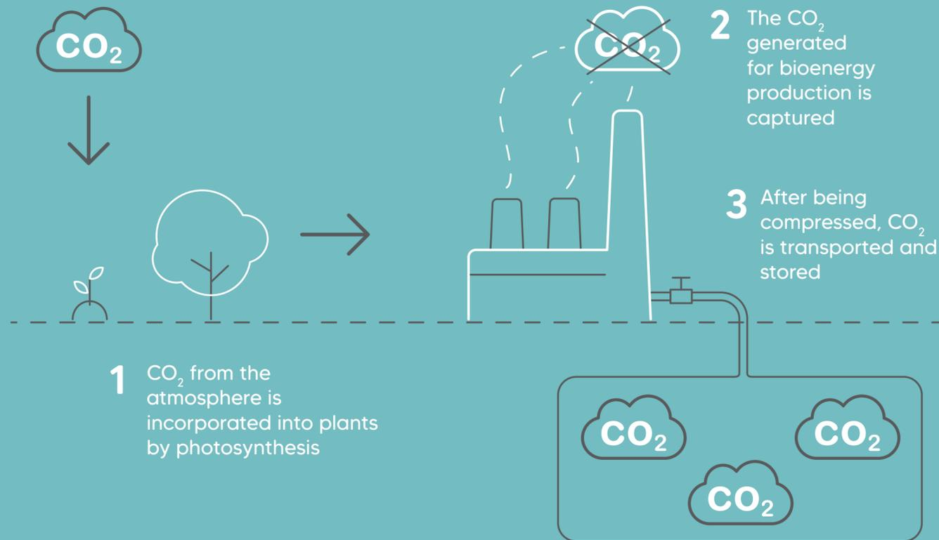
The BECCS process starts with the carbon arrest by vegetation with the duty of originating the bioenergy production. The CO<sub>2</sub> in the air is employed during photosynthesis.
