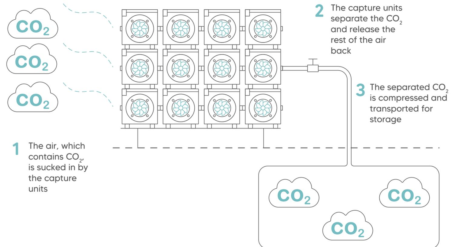
The direct air capture process with CCS, known as DACCS or DAC, is a relatively new technology, consisting of capture units drawing the air.
